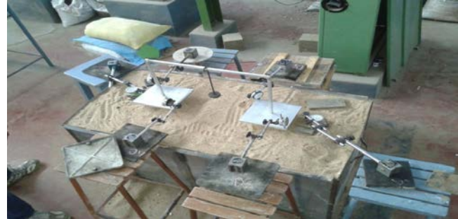
Fig.1 Photograph of Instrumented Model frame setup
